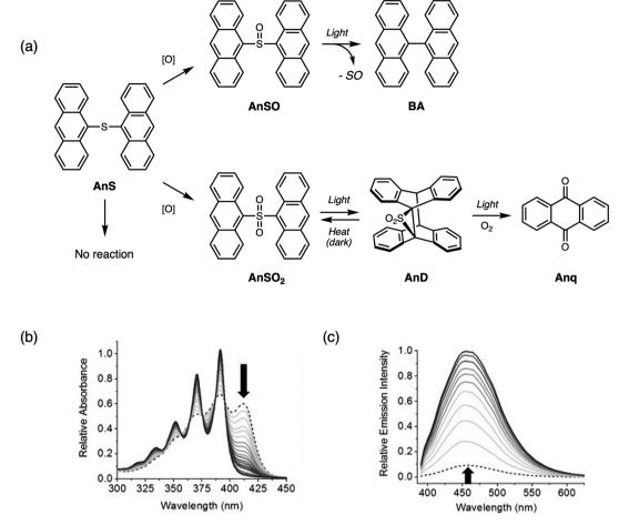
Fig. 12 (a) Different photochemical pathways of sulfur-bridged anthracene dimers  $AnSO_n$  (n = 0-2) depending on the oxidation state. Changes in the (b) UV-vis absorption and (c) emission spectra when AnSO is irradiated with UV light in  $CH_2Cl_2$ . Adapted with permission from ref. 64. Copyright 2013 Wiley.
