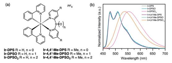
Fig. 16 (a) Structures of Ir(III) complexes  $Ir-DPSO_n$  and  $Ir-Me-DPSO_n$  (n=0-2) reported by our group. (b) PL spectra of the Ir(III) complexes in  $CH_2Cl_2$  solution ( $\lambda_{ex} = 390$  nm). Adapted with permission from ref. 82. Copyright 2017 American Chemical Society.
