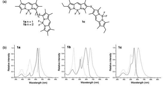
Fig. 2 (a) Structures of  $\alpha$ - or  $\beta$ -sulfide-bridged 1a and 1c and  $\alpha$ -disulfide-bridged 1b BODIPY dimers reported by Bröring. (b) UV-vis absorption (solid line), emission (dashed line) and excitation (dotted line) spectra of the dimers in CH<sub>2</sub>Cl<sub>2</sub>. Adapted with permission from ref. 29. Copyright 2013 Wiley.
