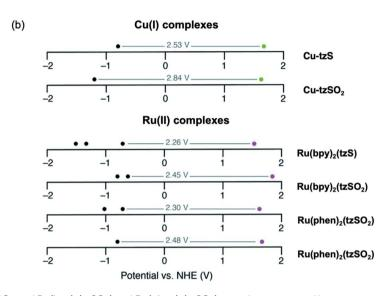
Fig. 19 (a) Structures of Cu-tzSO<sub>n</sub> and  $Ru(bpy)_2(tzSO_n)$  and  $Ru(phen)_2(tzSO_n)$  complexes reported by our group (n = 0, 2). (b) Redox potentials of Cu(i) and Ru(ii) complexes with reductive (black dots) and oxidative (green or purple dots) potentials illustrated. Adapted with permission from ref. 95. Copyright 2019 Royal Society of Chemistry.
