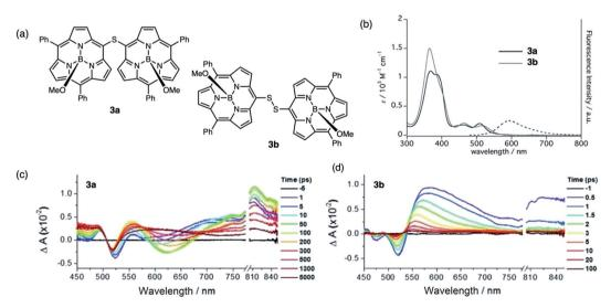
Fig. 4 (a) Structures of sulfide-bridged **3a** and disulfide-bridged **3b** subporphyrin dimers reported by Kim and Osuka. (b) UV-vis absorption (solid) and fluorescence (dashed) spectra of **3a** (black) and **3b** (gray) in  $CH_2Cl_2$ . (c and d) Transient absorption spectra of **3a** and **3b** in toluene ( $\lambda_{exc} = 490$  nm). Adapted with permission from ref. 35. Copyright 2016 Wiley.
