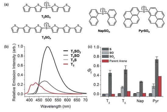
Fig. 7 (a) Structures of sulfur-bridged bithiophene  $T_2SO_n$ , terthiophene  $T_3SO_n$ , naphthalene NapSO<sub>n</sub> and pyrene PyrSO<sub>n</sub> dimers (n=0-2) reported by our group. (b) Emission spectra of  $T_3SO_n$  and  $T_3$  in  $CH_2Cl_2$ . (c) Photoluminescence quantum yields ( $\Phi_t$ ) of sulfur-bridged dimers with increasing oxidation states, in comparison to parent arenes. Adapted with permission from ref. 45. Copyright 2013 American Chemical Society.
