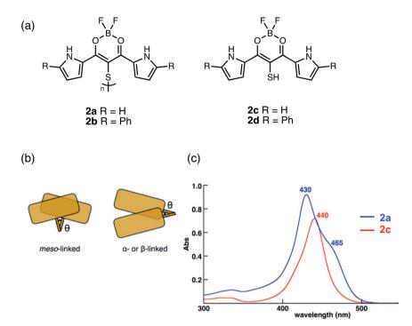
Fig. 3 (a) Structures of *meso*-disulfide-bridged boron dipyrroyldiketone dimers 2a and 2b and monomers 2c and 2d reported by Maeda. (b) Cartoon representation showing how *meso*-linked chromophores have greater areas of overlap compared to α- or β-linked dimers. (c) UV-vis absorption spectra of dimer 2a (blue) compared to monomer 2c (red) in  $CH_2Cl_2$ . Adapted with permission from ref. 33. Copyright 2017 American Chemical Society.
