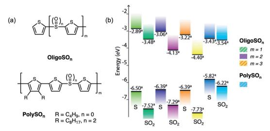
Fig. 10 (a) Structures of thiophene-based oligomers  $OligoSO_n$  and polymers  $PolySO_n$  containing a sulfur bridge (n = 0, 2) reported by our group. (b) Calculated frontier energy levels obtained from cyclic voltammetry measurements and UV-vis absorption spectra. Adapted with permission from ref. 49. Copyright 2017 American Chemical Society.
