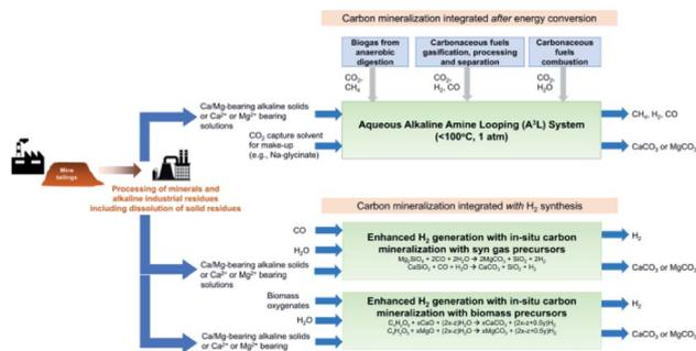
Fig. 5 Conceptual solvent-based capture and concurrent mineralisation. Image from Gadikota *et al.*, 2021.<sup>100</sup>
