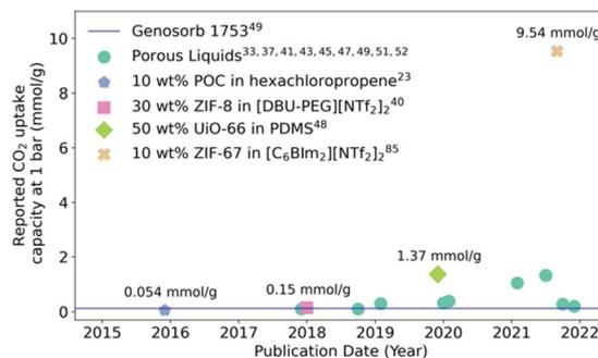
Fig. 5 Reported CO<sub>2</sub> uptake capacities in porous liquids at ca. 1 bar and ca. 298 K over time. A selection of the significant developments are highlighted to show the acceleration in progress.
