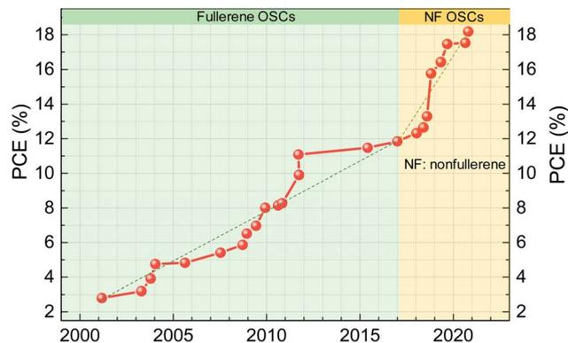
Fig. 1 Power conversion efficiency evolution of organic solar cells (data extracted from the NREL Best Research-Cell Efficiency Chart).<sup>31</sup> The dashed line is a guide for the eye to show the approximate slope of efficiency increase.
