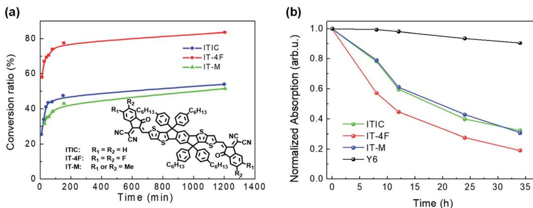
Fig. 6 (a) Plots of the NFA conversion ratio calculated from  $^1\text{H}$  NMR spectra as a function of reaction time with an ethanolamine : acceptor ratio of 4 : 1 at room temperature; (b) plots of the normalized absorption intensity of the main peak as a function of reaction time. Reproduced from ref. 45 with permission from the American Chemical Society, copyright [2020].
