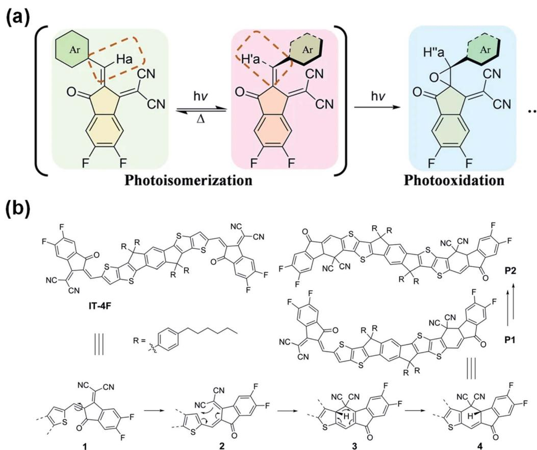
Fig. 9 (a) Photochemical reaction of NFAs; (b) mechanism of the photodegradation of IT-4F; reproduced from ref. 76 with permission from the Nature Publishing Group, copyright [2021]. Reproduced from ref. 77 with permission from the Wiley, copyright [2021].
