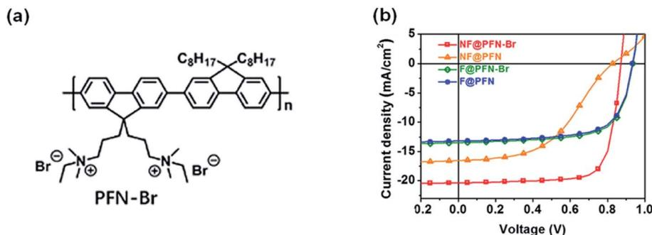
Fig. 18 (a) Chemical structure of PFN-Br. (b)  $J$ - $V$  characteristics of fullerene and nonfullerene OSCs with a PFN or PFN-Br interface, respectively. Reproduced from ref. 87 with permission with Elsevier, copyright [2020].
