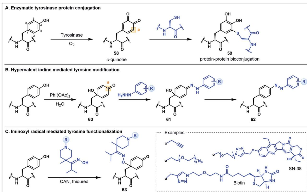
Fig. 9 Tyr functionalization using non-conventional umpolung strategies. (A) Tyr–Cys bioconjugation strategy using an enzymatically activated *o*-quinone intermediate. (B) Tyr dearomatization–rearomatization functionalization using phenyl hydrazine nucleophiles. (C) Tyr functionalization using iminoxyl radicals; CAN = ceric ammonium nitrate.
