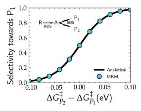
Fig. 4 Selectivity predictions in a model reaction network consisting of a rate determining step (RDS) followed by a selectivity determining step (SDS) leading to the two products,  $P_1$  and  $P_2$ . Cyan points show the results in the selectivity towards  $P_1$  ( $S_{P_1}$ ) resulting from a microkinetic model (MKM), with  $S_{P_1}$  calculated via eqn (8), while the solid black line represents the same selectivity calculated from the analytical eqn (9).
