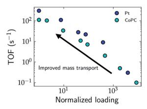
Fig. 2 Estimated TOF for the HER and CO<sub>2</sub>RR on Pt (blue) and CoPc (cyan) electrodes, respectively as a function of the normalized catalyst loading. Decreasing the catalyst loading can lead to improved mass transport and limit due to mass transport limitations even at these low loadings. While the TOF of CoPc reaches an upper limit at low loadings, the TOF for Pt does not reach an obvious upper limit due to mass transport limitations even at these low loadings.
