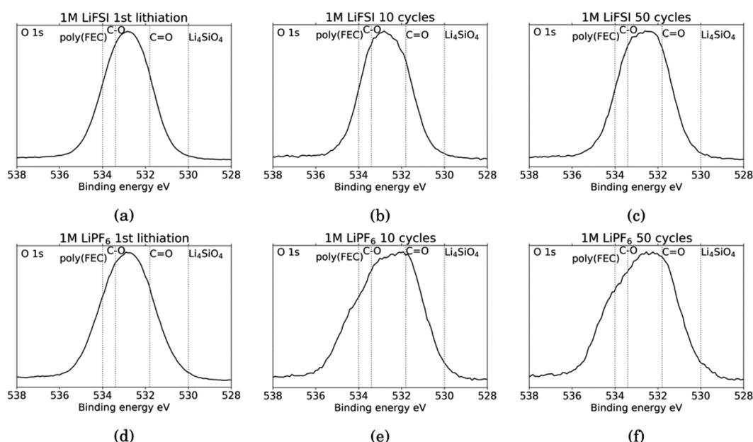
**Fig. 6** O 1s spectra for Si electrodes cycled to 1st lithiation, cycle 10 and cycle 50 in LiFSI (a–c) respectively, and in LiPF<sub>6</sub> (d–f) respectively.
