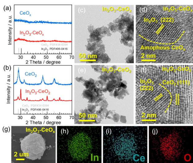
**Fig. 1** (a) XRD patterns of  $\text{CeO}_x$  and  $\text{In}_2\text{O}_3\text{--CeO}_x$ , (b) XRD patterns of  $\text{CeO}_2$  and  $\text{In}_2\text{O}_3\text{--CeO}_2$ , (c and d) HR-TEM image of  $\text{In}_2\text{O}_3\text{--CeO}_x$  and (e and f) HR-TEM image of  $\text{In}_2\text{O}_3\text{--CeO}_2$ . (g–j) The corresponding EDX elemental mapping of  $\text{In}_2\text{O}_3\text{--CeO}_x$ .
