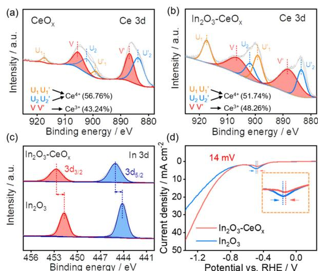
**Fig. 2** Ce 3d XPS spectra of (a)  $\text{CeO}_x$  and (b)  $\text{In}_2\text{O}_3\text{--CeO}_x$ ; (c) In 3d XPS spectra of  $\text{In}_2\text{O}_3\text{--CeO}_x$  and  $\text{In}_2\text{O}_3$ ; and (d) LSVs of  $\text{In}_2\text{O}_3$  and  $\text{In}_2\text{O}_3\text{--CeO}_x$  in  $\text{CO}_2$ -saturated 0.5 M  $\text{KHCO}_3$  at a scan rate of  $50\text{ mV s}^{-1}$ .
