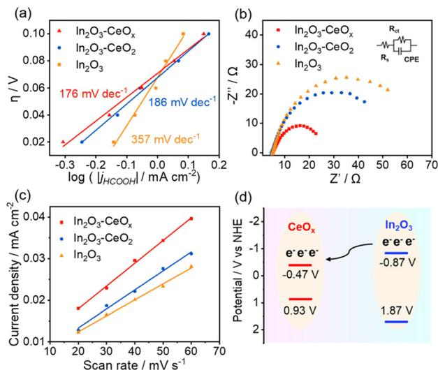
**Fig. 4** Advantages of  $\text{In}_2\text{O}_3\text{-CeO}_x$  for  $\text{CO}_2$  reduction. (a) Tafel plots, (b) Nyquist plots (inset: equivalent circuit), (c) linear fitting of double-layer capacitive currents versus scan rates to estimate the ECSA of  $\text{In}_2\text{O}_3\text{-CeO}_x$ ,  $\text{In}_2\text{O}_3\text{-CeO}_2$  and  $\text{In}_2\text{O}_3$ , and (d) schematic illustration of the charge transfer in  $\text{In}_2\text{O}_3\text{-CeO}_x$ .
