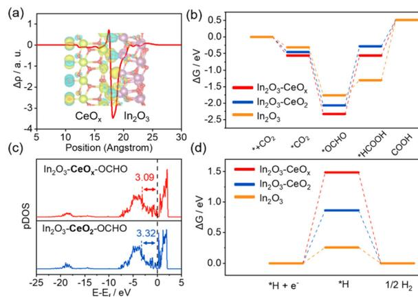
**Fig. 5** DFT calculations. (a) Charge density difference and charge displacement curves of  $\text{In}_2\text{O}_3\text{-CeO}_x$ ; purple, yellow, and red spheres represent In, Ce, and O atoms, respectively. (b) Gibbs free-energy diagrams of  $\text{CO}_2$ -to-formate. (c) In-5p p-DOS of  $\text{In}_2\text{O}_3\text{-CeO}_x$  and  $\text{In}_2\text{O}_3\text{-CeO}_2$  after adsorbing  $^*\text{OCHO}$ . (d) Gibbs free-energy diagrams of the HER.
