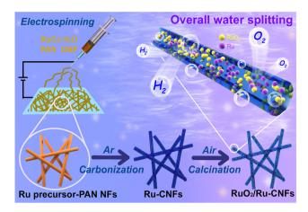
Scheme 1 Schematic diagram of the fabrication of RuO<sub>2</sub>/Ru-CNFs.
