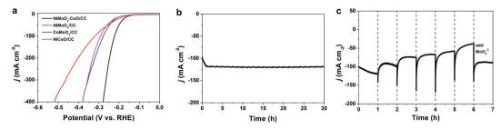
Fig. 2 (a) LSV curves of NiMoO<sub>4</sub>-CoO/CC, NiMoO<sub>4</sub>/CC, CoMoO<sub>4</sub>/CC, and NiCoO/CC. (b) J-t curve of NiMoO<sub>4</sub>-CoO/CC in 1.0 M KOH. (c) J-t curve of NiMoO₄-CoO/CC obtained by renewing the electrolyte every 1 hour.
