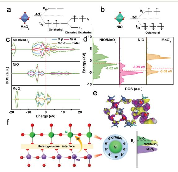
Fig. 5 (a) 4d orbital energy levels of Mo<sup>4+</sup> and the Jahn-Teller effect, (b) schematic electronic configuration of the Ni cations in NiO, (c) DOS and PDOS and (d) d-band center level of NiO, MoO<sub>2</sub> and NiO/MoO<sub>2</sub>, respectively, (e) electron density difference of the NiO/MoO<sub>2</sub> interface, (f) schematic illustration of the electron transfer of the Mo and Ni atom, and the valence band of NiO, MoO2 and NiO/MoO2.
