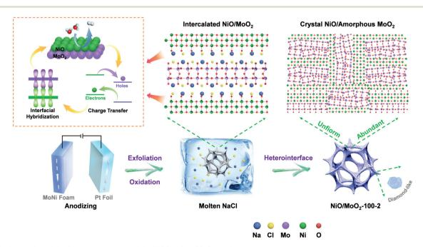
Scheme 1 Illustration of the fabrication process of the NiO/MoO<sub>2</sub>-100-2 sample.
