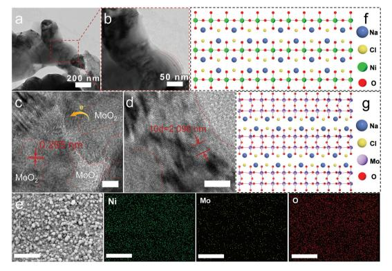
Fig. 2 Structural analysis of NiO/MoO<sub>2</sub>-100-2. (a and b) TEM images. (c and d) HRTEM images, c, scale bar: 2 nm; d, scale bar, 3 nm. The red lines denote the crystal/amorphous interfaces. (e) SEM mapping, scale bar: 10 μm. Atomic structures of (f) NiO and (g) MoO<sub>2</sub>.
