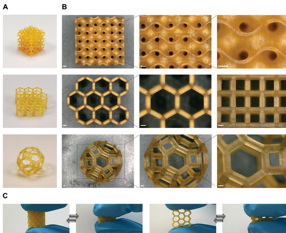
**Fig. 3** High resolution 3D printing with P1/P2 85/15, w/w dual-polymer resin. (A and B) Pictures (A) and corresponding microscopy images (B) of three 3D printed objects with complex architectures. Scale bars 500  $\mu$ m. (C) The 3D printed objects showing high elasticity indicated by finger compression.
