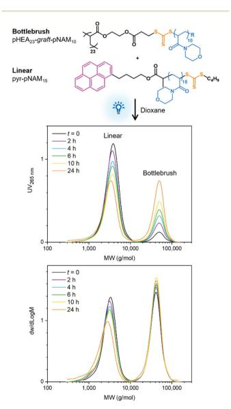
Fig. 2 SEC data shows exchange of pHEA23-graft-pNAM10 grafts for pyrene-functional linear pNAM<sub>15</sub> chains. Analysis was conducted in CHCl<sub>3</sub> with DRI and UV<sub>265 nm</sub> detection and PMMA calibration.
