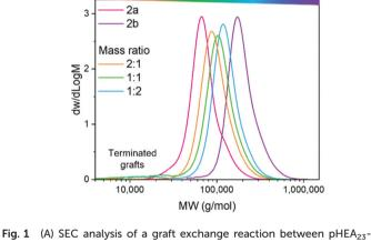
graft-pNAM<sub>10</sub> and pHEA<sub>23</sub>-graft-pNAM<sub>87</sub>. (B) SEC analysis of pHEA<sub>133</sub>- $\textit{graft}\text{-pNAM}_{8}$ ,  $pHEA_{133}\text{-}\textit{graft}\text{-pNAM}_{29}$ , and the products of exchange reactions carried out using 2:1, 1:1 and 1:2 mass ratios of the two polymers. Analysis was performed in DMF with DRI detection and PMMA calibration
