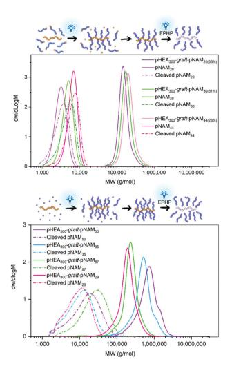
Fig. 4 SEC data of grafts cleaved off polymers synthesised via grafting of linear pNAM to pCTA $_{300}$  (top) and the Z group approach (bottom). Analysis was conducted in DMF with DRI detection and PMMA calibration.
