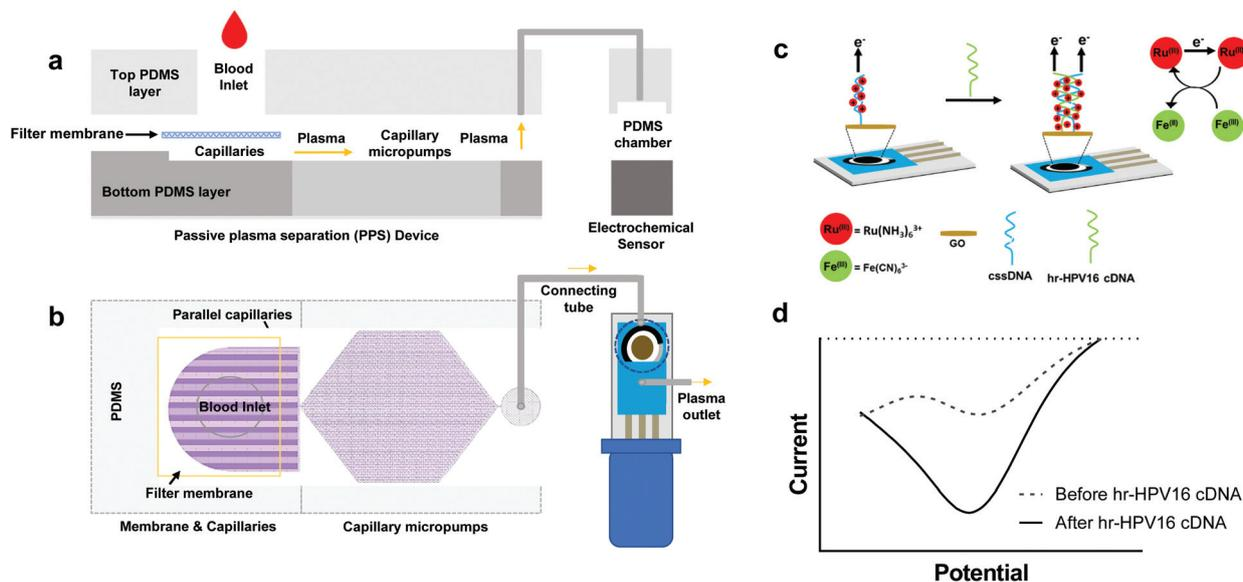
**Fig. 1** Overview and working mechanisms of IMEAC. Side view (a) and top view (b) of the IMEAC device that integrates two main modules: PPS for plasma isolation and an electrochemical biosensor. (c) Working principle of the electrochemical sensor for hr-HPV16 cDNA detection. (d) A sample graph extracted from IMEAC showing the presence of hr-HPV cDNA in the extracted plasma sample.
