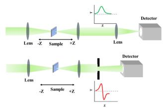
Schematic representation of the Z-scan setup used for the NLO
