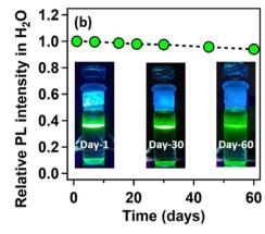
Fig. 4 Water stability of the MAPbBr $_3$ @lead laurate core-shell NC system. (a) Comparative PL spectra of the MAPbBr $_3$ @lead laurate core-shell NC system in water, recorded on day-1, day-30, and day-60 upon exciting at 400 nm. (b) Relative change in PL intensity with the progress in days of the MAPbBr $_3$ @lead laurate core-shell NC system in water under UV (365 nm) for day-1, day-30, and day-60 are given in the inset.
