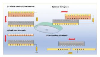
Fig. 1 Fundamental modes for TENG operation for the (a) vertical contact/separation mode, (b) lateral sliding mode, (c) single electrode mode, and (d) freestanding mode.
