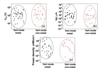
Fig. 7 Comparison of the responses summarized in Tables 1 and 2 for the vertical mode of operation for metal-based devices (in black) and no-metal-based devices (in red) for  $V_{\rm OC}$  (a),  $I_{\rm SC}$  (b), and power output (c).
