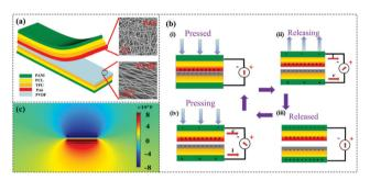
Fig. 2 (a) Disposition of the conducting layer and active triboelectric electrospun nets. (b) Scheme of the operation mode of the vertical contact-separation method in a complete cycle of contact separation and (c) simulation of the potential distribution between two triboelectric materials. Reprinted from ref. 57, Copyright (2019), with permission from
