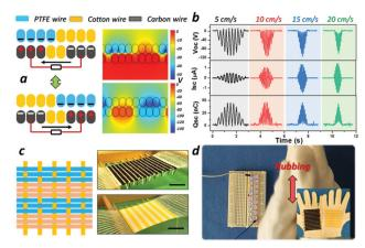
(a) Scheme of the free-standing mode PTFE grating textile and interdigital carbon textile electrode for horizontal motion, (b) measurements of Voc, Isc, and Qsc under operation, (c and d) photographs of the electrode and sliding textile under operation with commercial blue LEDs. Reprinted from ref. 86. Copyright (2018), with permission from Elsevier.
