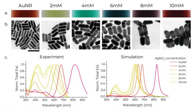
Fig. 1 Synthesis of Au/AgNRs with varying shell thickness. (a) Variation of colour of Au/AgNR suspensions grown with different concentrations of Ag<sup>+</sup> ions. (b) Transmission electron micrographs of Au/AgNRs with Ag shells of different thicknesses. The concentration of Ag<sup>+</sup> in the growth solution is shown at the top. All images are to scale. Scale bar: 100 nm. (c) Experimental and theoretical extinction spectra of the AuNRs and Au/AgNRs with varying shell thickness.
