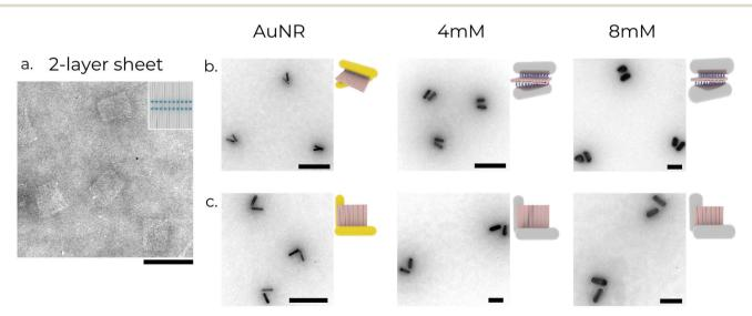
Fig. 3 Structural characterisation of chiral metamolecules. (a) Transmission electron micrograph of the 2-layer sheet DNA origami structures. (b) and (c) X- and L-shaped left-handed chiral structures assembled using three varieties of nanorods, respectively. The concentration of AgNO<sub>3</sub> used to synthesise the nanorods used for the structures is shown above the images. All scale bars: 100 nm.
