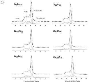
Fig. 6  $^{11}$ B MAS NMR spectra for the  $Ca_xZn_y$  glass series. (a) Stacked <sup>11</sup>B MAS NMR for each glass composition; and (b) spectral deconvolution, with the dashed line indicating the applied fit.
