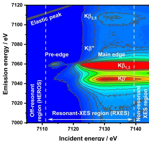
Fig. 1 RXES plane of FeCl<sub>3</sub> with all important features and HEROS, RXES, and nXES regions marked.
