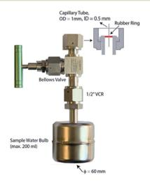
Fig. 2 Water sample container for <sup>3</sup>He ingrowth analysis at the IAEA.
