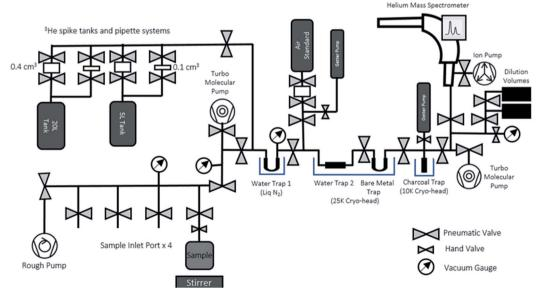
Fig. 4 A schematic diagram of the helium analytical system for the <sup>3</sup>He ingrowth method.
