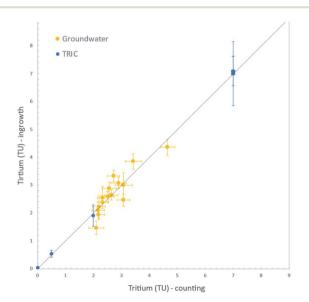
Fig. 7 Comparison of tritium analysis on groundwater samples by decay counting and by the  $^3$ He ingrowth method. A 1:1 line is shown for reference. Results of analysis on the TRIC analysis are also shown.
