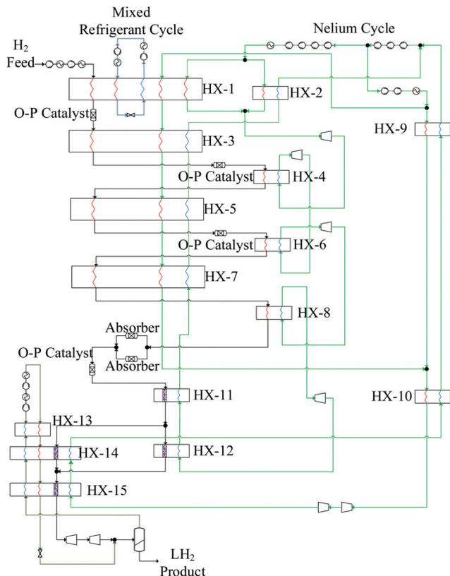
Fig. 8 Process block diagram for IDEALHY project.
