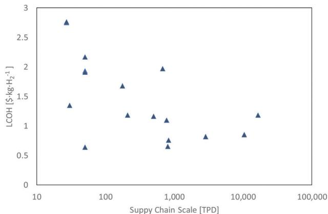
Fig. 18 Liquefaction cost component of the LCOH studies shown in Fig. 17 as a function of the supply chain scale.
