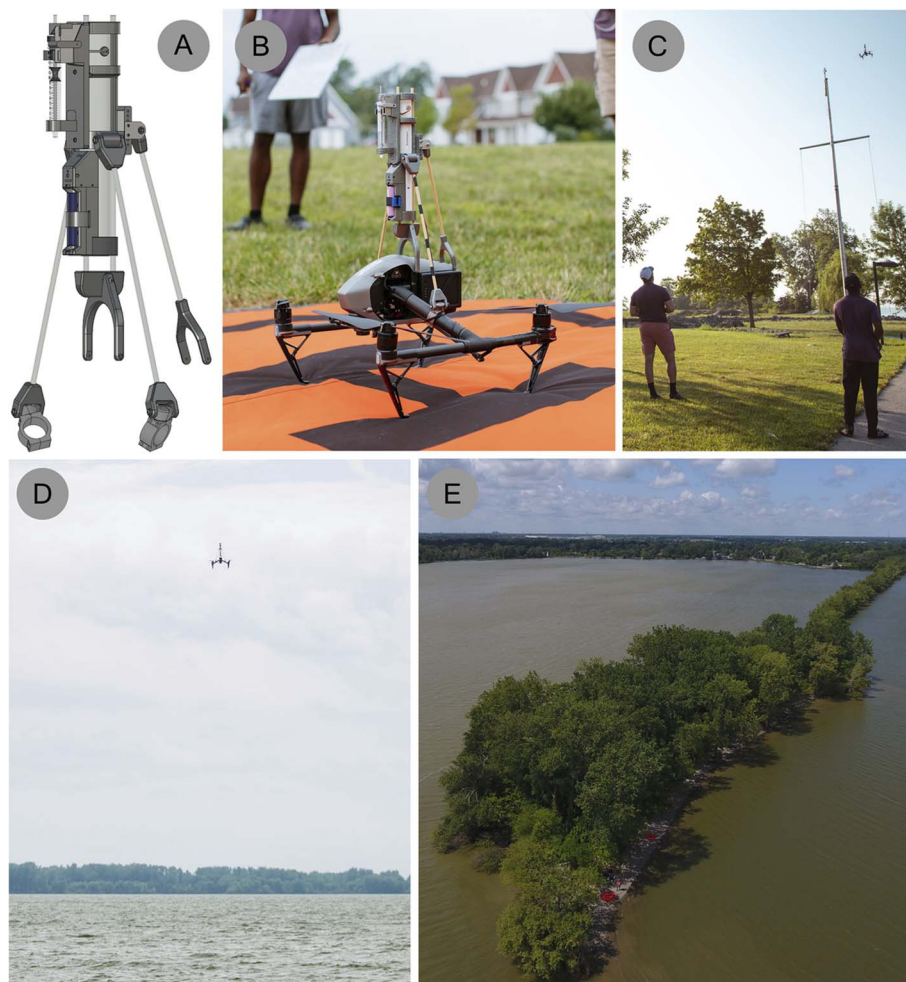
Fig. 1 (A) Engineering model of the AirDROPS package. (B) The AirDROPS attached to the DJI Inspire 2 platform. (C) Intercomparison flight of the AirDROPS adjacent to the sonic anemometer mounted on the flagpole. (D) Sampling mission at GLMS, 10 m above the surface of the water. (E) Drone image and aerial view of the sampling location at LE to the right of the point in the image.
