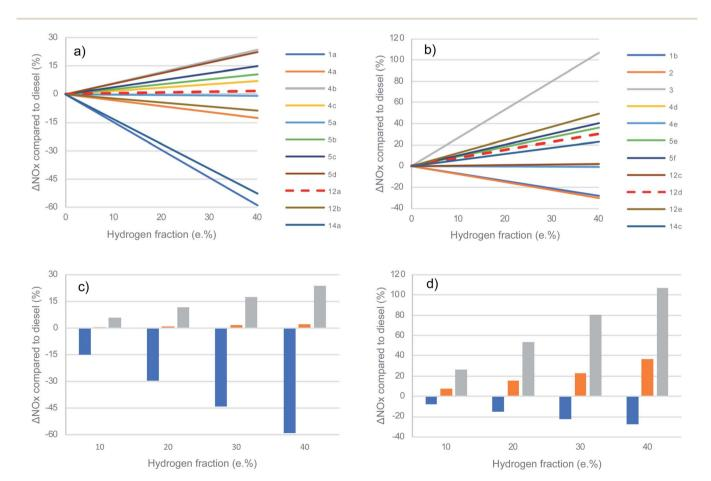
Fig. 1 Meta-analysis of effect on  $NO_x$  emissions for H2D combustion in large diesel engines for different H2D fuel compositions. (a) 0–30% low load case (b) 50–100% high load case. Numbers in the legend correspond to datasets in Table 1. The median dataset is presented as a red dashed line. (c) Worst (grey), median (orange) and best-case (blue)  $NO_x$  scenarios for 0–30% load (d) worst (grey), mean (orange) and best-case (blue) scenarios for 50–100% load.
