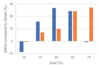
Fig. 2 NO<sub>x</sub> emissions from combustion of H2D dual fuel of composition 40 e% hydrogen, for engine loads 10-40%. Raw data for the engine with EGR (blue) is taken from dataset 4 (see Table 1). Raw data for the engine without EGR (orange) is taken from dataset 5 (see Table 1).
