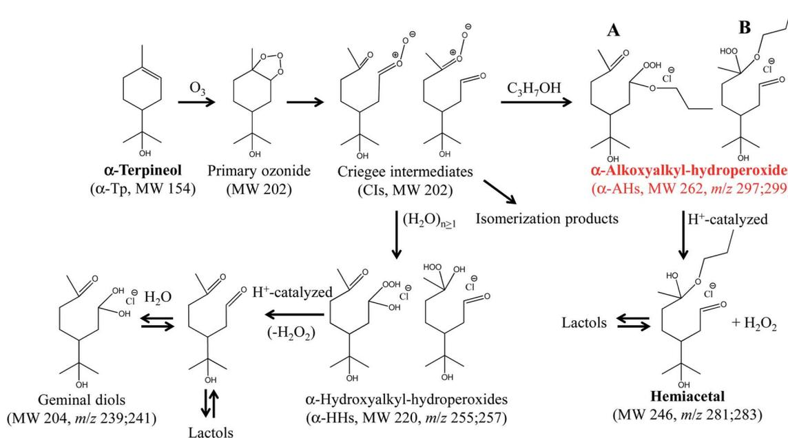
Scheme 1 The formation and decomposition of  $\alpha$ -AHs (A; secondary  $-\text{OOH}$ , B; tertiary  $-\text{OOH}$ ) and  $\alpha$ -HHs derived from ozonolysis of  $\alpha$ -terpineol in 1-propanol : water (1 : 1 = vol/vol) solutions. The likely isomers are shown.<sup>16</sup>
