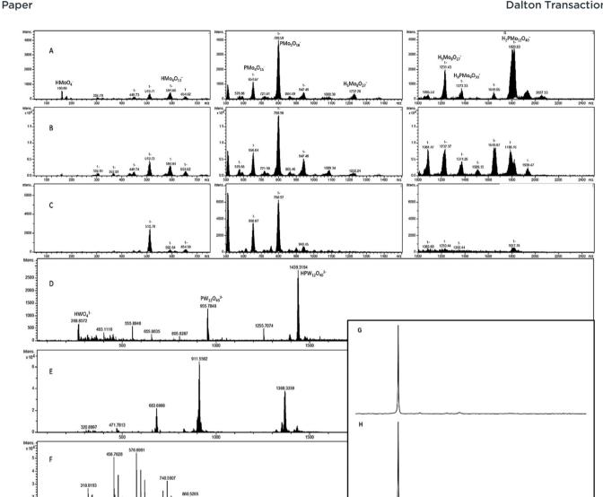
Fig. 10 Mass and NMR spectra of POM-diglycine complexes dissolved in different media. Diglycine-PMo complex 2 (3:1) (1.5 mM) 2 was dissolved in (A) 0.2 M HCl, (B) water, and (C) phosphate buffer (5 mM, pH 6.5). Diglycine-PW complex (3:1) (14 uM) dissolved in (D) 0.2 M HCl, (E) water, and (F) phosphate buffer (5 mM, pH 6.5). (G) and (H) 31P NMR spectra of phoshomolybdate at pH 6 with diglycine (compound 2) and without diglycine respectively.
