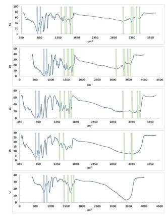
Fig. 9 FT-IR spectra of compounds 2, 3, 4, 6, and 7. Signals corresponding to bonds in the PMo particle are indicated in blue, signals corresponding to diglycine bonds are indicated in green.
