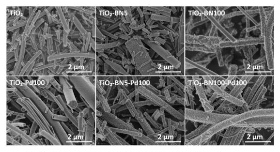
Fig. 2 SEM images of TiO<sub>2</sub>, TiO<sub>2</sub>-BN5, TiO<sub>2</sub>-BN100, TiO<sub>2</sub>-Pd100, TiO<sub>2</sub>-BN5-Pd100 and TiO<sub>2</sub>-BN100-Pd100 nanocomposites.
