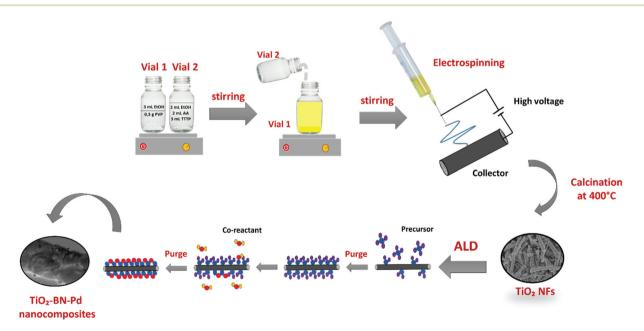
Fig. 1 Illustration of the steps for the preparation of nanocomposites. In the first step we prepared the polymeric solution, then electrospinning was performed. The collected nanofibers were then calcined before the ALD process.
