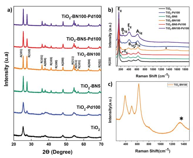
Fig. 3 (a) XRD data (b) Raman spectra of bare TiO<sub>2</sub> and synthesized nanocomposites and (c) zoom on Raman spectra of TiO<sub>2</sub>-BN100.
