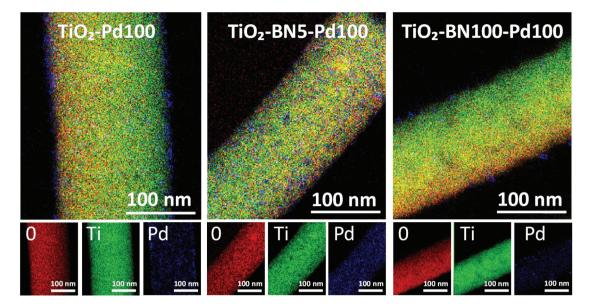
Fig. 5 EDS elemental mapping of TiO<sub>2</sub>-Pd100, TiO<sub>2</sub>-BN5-Pd100 and TiO<sub>2</sub>-BN100-Pd100 nanofibers.
