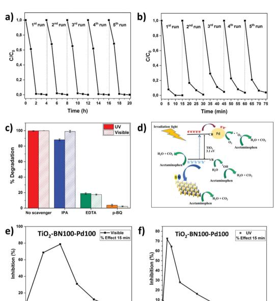
Fig. 11 Recycling test of  $TiO_2$ -BN100-Pd100 under (a) visible and (b) UV irradiation; (c) scavenger plot for determining reactive species in the degradation of ACT by  $TiO_2$ -BN100-Pd100; (d) mechanism of ACT degradation by  $TiO_2$ -BN100-Pd100; inhibition of luminescence of *V. fischeri* marine bacteria during ACT photocatalysis after 15 min exposure between the bacterial strain and the degradation solution under (e) visible and (f) UV irradiation.
