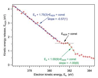
Fig. 7 Kinetic energy release in the dissociation events, based on the median momentum of the NH<sub>2</sub><sup>+</sup> ions
