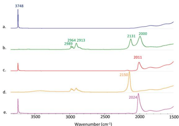
**Fig. 1** Diffuse reflectance infrared Fourier transform spectra of SBA-15<sub>700</sub> (a),  $\equiv\text{SiOAl}(\text{Cp}^*\text{IrH}_3)_2$  **2-s** (b), **Ir-Al/SiO<sub>2</sub>** (c),  $\text{Cp}^*\text{IrH}_4$  physisorbed on SBA-15<sub>700</sub> (d) and **Ir/SiO<sub>2</sub>** (e) recorded on powder materials under argon.
