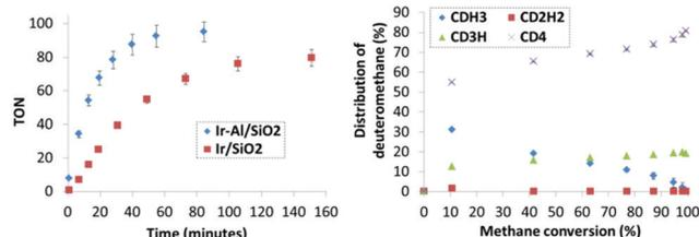
Fig. 4 Monitoring catalytic H/D exchange of methane. Left: Turnover number as a function of reaction time for catalysts Ir-Al/SiO<sub>2</sub> and Ir/SiO<sub>2</sub> at 250 °C and 0.67 mol% Ir surface sites. Right: Distribution of deuteromethanes as a function of CH<sub>4</sub> conversion for Ir-Al/SiO<sub>2</sub>.
