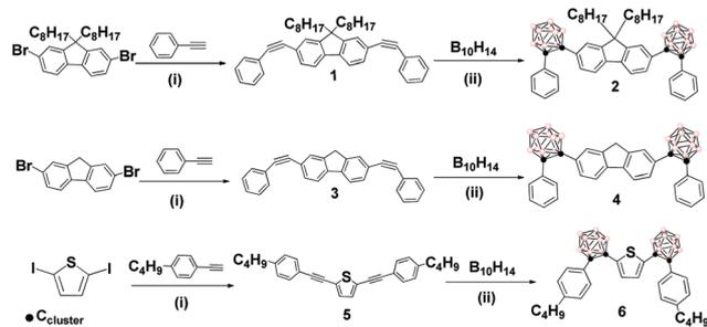
**Scheme 1** Synthesis of fluorene- and thiophene-based  $\pi$ -conjugated systems linked to *o*-carborane clusters: (i) Pd(PPh<sub>3</sub>)<sub>2</sub>Cl<sub>2</sub>, CuI, TEA and toluene (1:9 v/v); (ii) 5 eq. Et<sub>2</sub>S, toluene, 72 h, and 110 °C.
