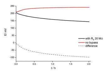
Fig. 6 Dependence of open circuit potential on time for a potassium-selective ISE, non-bypassed (red line) and bypassed (black line) by zinc wire and resistor  $R_{\rm b}$  = 20 M $\Omega$ . Dashed line: difference of potentials in the presence and absence of bypass.
