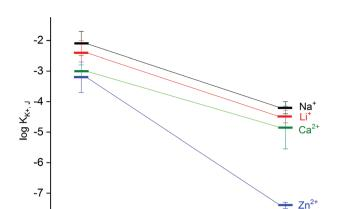
Fig. 5 Effect of applied bypass resistance on the selectivity of potassium-selective ISE, mean value of logarithm of selectivity coefficient  $\pm$  SD is shown, the value presented was determined for activity range from  $10^{-3}$  to 0.1 M using experimental slopes.
