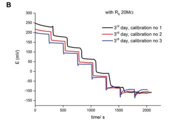
Fig. 4 (A) Selected potentiometric calibration plots for potassium-selective ISE, bypassed by zinc wire and resistor  $R_{\rm b} = 20~{\rm M}\Omega$ , third calibration for each consecutive day is presented: (**II**) 1st day, (**O**) 2rd day (C) 3rd day. (B) Time traces for the sequential calibrations of the 3rd day.
