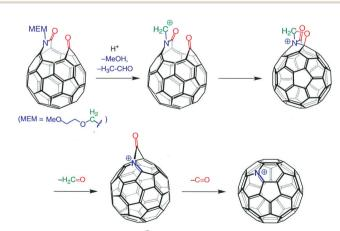
Fig. 2 Formation of heterofullerene  $C_{59}N$ .
