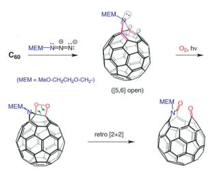
Fig. 1 Azafulleroid conversion to "holey bucky".6
