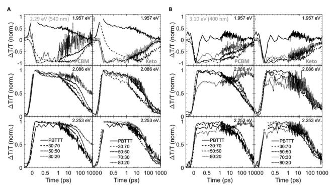
Fig. 5 Spectral transient absorption cuts taken at different energies (1.957 eV: top panels; 2.086 eV: middle panels; 2.253 eV: bottom panels), photoexcited at 2.29 eV (540 nm) (A) and 3.1 eV (400 nm) (B). Data for PCBM-based binaries are shown in the left panels; those for ketolactam systems
