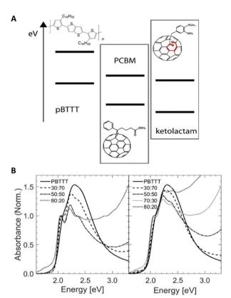
Fig. 1 (A) Schematic representation of the energy levels of the polymer (PBTTT) and fullerene acceptors, i.e., PCBM and ketolactam fullerene, used here to scrutinize the power of temperature/composition phase diagrams for property mapping of corresponding blends. Chemical structures are shown as insets. (B) UV-vis spectroscopy data of a range of blends of PCBM:PBTTT (left) and ketolactam:PBTTT (right; compositions given as mass ratio), and for comparison: neat PBTTT.
