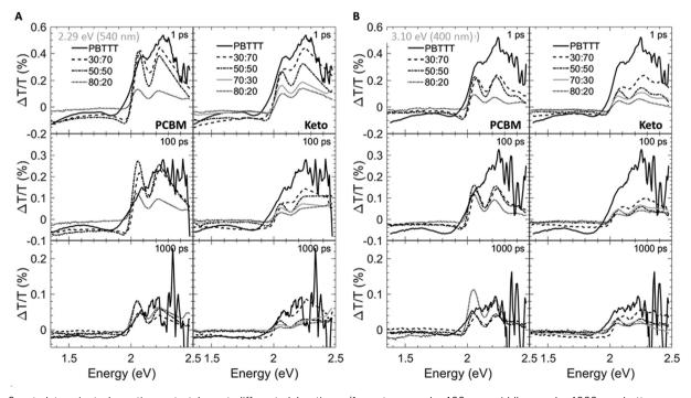
Fig. 4 Spectral transient-absorption cuts taken at different delay times (1 ps: top panels; 100 ps: middle panels; 1000 ps: bottom panels) for fullerene: PBTTT blends photoexcited at 2.29 eV (540 nm) (A) and 3.1 eV (400 nm) (B). Data for PCBM-based binaries are shown in the left panels; those for **ketolactam** systems on the right.
