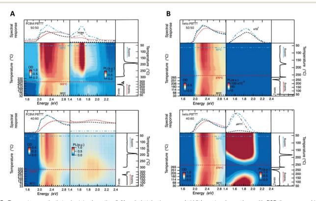
Fig. 3 Temperature-resolved steady-state absorption (left) and photoluminescence (middle) spectra shown along with DSC thermograms (right), obtained at 20 °C min<sup>-1</sup> heating/cooling for DSC, and at 20 °C min<sup>-1</sup> heating (10 °C min<sup>-1</sup> cooling) for absorption and PL for (A) 50:50 and 40:60 PCBM: PBTTT (top and bottom, respectively), and (B) the equivalent ketolactam: PBTTT binaries
