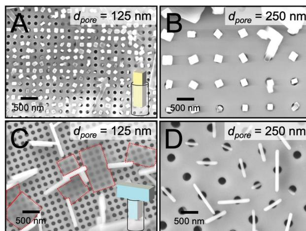
Fig. 3 TIPS-PY crystals ( $n = 1$ ) on nanoconfining scaffolds with cylindrical nanopores ( $m = 1$ ) for nanopore diameters of (A) 125 nm and (B) 250 nm. (C and D) Perylene crystals ( $n = 2$ ) deposited on the same  $m = 1$  scaffolds, respectively. Illustrations of crystal shapes and orientations within the nanopores are provided in A and C. Red dashed lines highlight crystals that nucleated on top of the scaffold for clarity.
