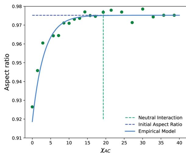
**Fig. 14** Aspect ratio (AR) as a function of the interaction parameter,  $\chi_{AC}$ , of newly created monomers on the solvophobic block. The neutral interaction point occurs when C particles can no longer distinguish between A and B beads, *i.e.* when  $\chi_{AC} = \chi_{BC}$ .
