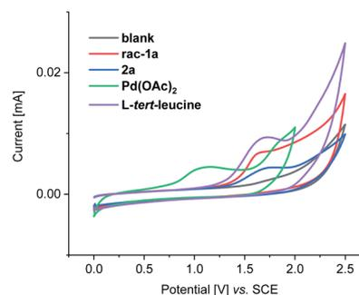
Fig. 4 Cyclic voltammogram of several reactants in AcOH with *n*Bu<sub>4</sub>NPF<sub>6</sub> (0.1 M) at 100 mV s<sup>-1</sup>.
