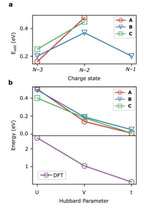
Fig. 5 (a) Addition energies from experimental stability diagrams for devices A–C. (b) The Hubbard parameters for the devices that reproduce these addition energies (upper panel) along with DFT calculations of these values (lower panel).
