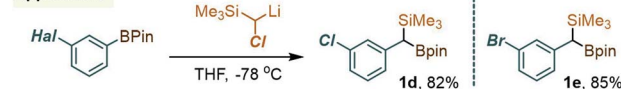
Scheme 2 Complementary deprotonation/quench approaches to the benzylic gem-Si/B core 1a . Approach A: (i) in hexane using 1.0 equiv. of n -BuLi at rt; (ii) with 3 equiv. of B(OMe) 3 , –78 °C to rt. Approach B: Li-TMP generated at –40 °C prior to addition of BnBpin at –78 °C. Approach C: lithiation of Me 3 SiCH 2 Cl with sec -BuLi/TMEDA followed by addition of Ar-Bpin.
