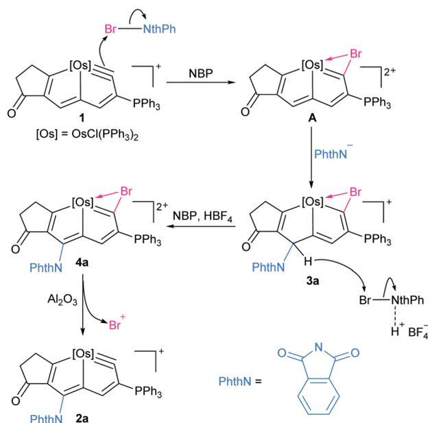
Scheme 3 Proposed mechanism for the direct amidation of metallaaromatics, [Os] = OsCl(PPh<sub>3</sub>)<sub>2</sub>.
