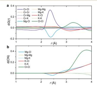
Fig. 3 Interpretation of the differential PDF. (a) Partial subcomponents of dG(r) from AIMD simulations. (b) Differential coordination number d(CN) for the solvent–solvent correlations, showing the difference between the cumulative coordination number in the  $CrCl_3$  loaded system and the pristine  $KCl-MgCl_2$  molten salt.
