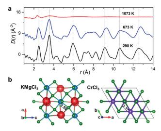
Fig. 1 Temperature-dependent PDF results. (a) X-ray reduced pair distribution functions, D(r), for the KCl-MgCl<sub>2</sub> salt mixture (50:50 mol%). (b) KMgCl<sub>3</sub> (Pnma) and CrCl<sub>3</sub> ( $P3_112$ ) crystal structures with highlighted Mg-Cl and Cr-Cl average bond lengths in Å. Color scheme: K, red; Mg, blue; Cr, purple; Cl, green. Vertical dashed lines in (a) are guides to the eye.
