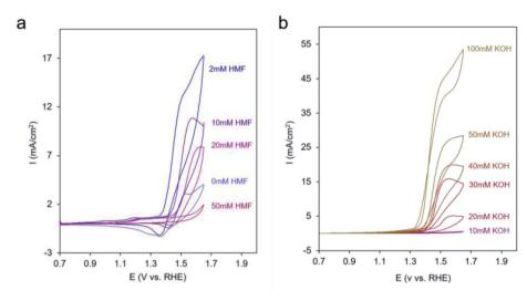
Fig. 5 CV cycles with Ni-MOF-74D under 10 mM KOH upon increasing the HMF concentration (a) and at 50 mM HMF with increasing the KOH concentration (b).
