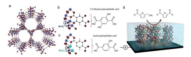
Fig. 1 Ni-MOF 74 contains cylinder shaped pores and chains of 5-coordinate Ni oxide units (a). The 2,5-dihydroxyterepthalic acid organic linker, will bind through both the carboxylate and alcohol units (b) and replacing it with 2-hydroxyterepthalic acid will result in defect sites of 4-coordinate Ni sites (c). We studied the effects of these defect sites with electrochemical and spectroscopic techniques, using the oxidation of HMF as a model reaction (d).
