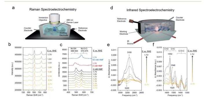
Fig. 6 Raman setup used for spectroelectrochemical measurements (a). Absolute (b) and difference spectra (c) illustrate that both \*OH and adsorbed HMF are necessary for the reaction mechanism in 10 mM KOH conditions. IR spectroscopy under the same conditions with the setup illustrated in (d) shows the adsorption of \*OH (e) and changes in surface bound HMF as it is oxidized to DFF (f).
