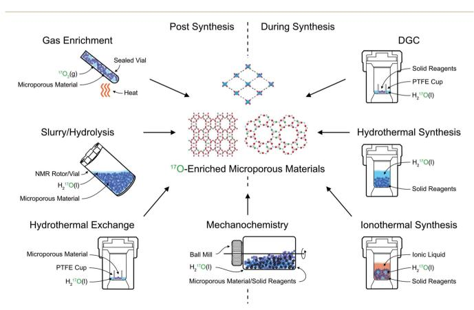
Fig. 2 Schematic showing approaches for <sup>17</sup>O enrichment of microporous materials during and post synthesis.
