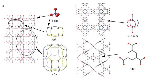
Fig. 1 (a) The structure of CHA zeolite showing the *d6r* and *cha* cage secondary building units (SBUs) with four-, six- and eight-membered rings highlighted. (b) The structure of the Cu-based MOF HKUST-1 (viewed down the (010) and (110) directions) showing the Cu "paddlewheel" dimer and benzene tricarboxylate (BTC) linker building units.
