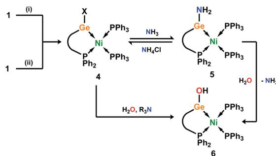
Scheme 3 Synthesis of halo-germylene Ni<sup>0</sup> complexes **4** and subsequent reactions with NH<sub>3</sub> and H<sub>2</sub>O. (i) 1.1NiX<sub>2</sub>·DME, 2Ph<sub>3</sub>P, 6Zn, THF, 2 h (X = Br); ~24 h (X = Cl); X = Cl and/or Br; (ii) 1Ni(cod)<sub>2</sub>, 2Ph<sub>3</sub>P, toluene, 1 h; X = Cl.
