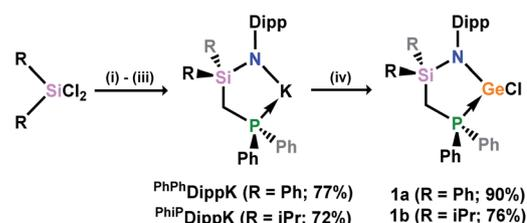
Scheme 1 The synthesis of phosphine-functionalised amine pro-ligands, their deprotonation, and subsequent synthesis of chloro-germylene complexes. (i) Ph<sub>2</sub>PCH<sub>2</sub>Li·TMEDA, hexane; (ii) DippN(H)Li, THF; (iii) KH, THF; (iv) GeCl<sub>2</sub>·dioxane, THF (yields in parentheses). Dipp = 2,6-<sup>i</sup>Pr<sub>2</sub>-C<sub>6</sub>H<sub>3</sub>.
