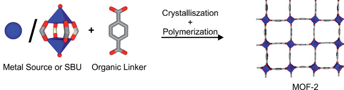
Fig. 1 (a) Schematic depiction of a range of conventional 2D materials. (b) 2D framework materials, their building blocks and synthetic procedures: (i) 2D polymers, (ii) 2D covalent-organic frameworks and (iii) 2D metal-organic frameworks.
