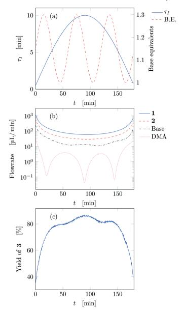
Fig. 3 Time variation of the input and output parameters for run 1 of Table 1: (a) instantaneous residence time and base equivalents; (b) species flowrate; (c) measured yield of the desired product.
