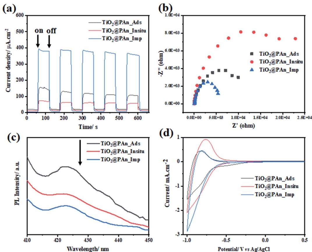
Fig. 12 (a) Transient photocurrent response ( $I-t$ ) curves; (b) EIS Nyquist plots under light irradiation; (c) the photoluminescence spectra (PL) measured at an excitation wavelength of 350 nm, and (d) cyclic voltammetry curves of  $\text{TiO}_2@PAN_{Insitu}$ ,  $\text{TiO}_2@PAN_{Ads}$ , and  $\text{TiO}_2@PAN_{Imp}$  photocatalysts.
