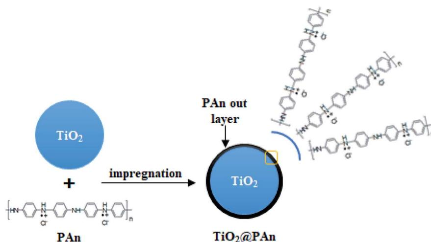
Fig. 1 Schematic illustration of  $\text{TiO}_2@PAn$  composite fabrication.
