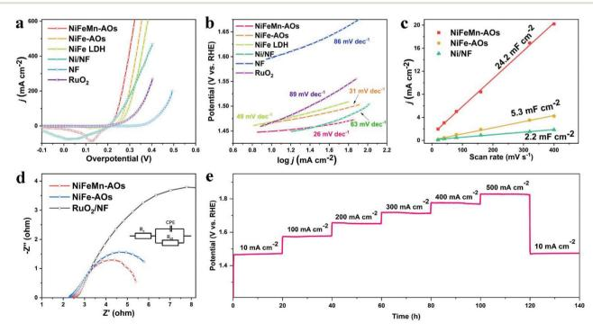
Fig. 3 The performance of the oxygen evolution reaction. (a) The LSV curves of various electrodes. (b) The Tafel plots calculated from polarization curves. (c)  $C_{\rm cl}$  values of Ni/NF, NiFe-AOs and NiFeMn-AOs. (d) EIS Nyquist plots of RuO<sub>2</sub>/NF, NiFe-AOs and NiFeMn-AOs electrodes with 250 mV overpotential. (e) Multi-chronopotentiometry curves of NiFeMn-AOs under various current densities.
