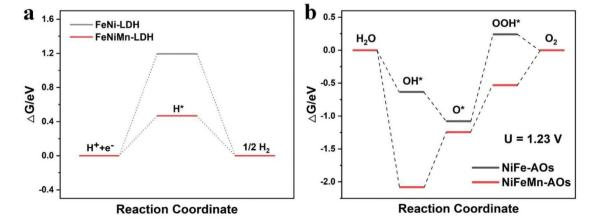
Fig. 6 (a) Gibbs free-energy diagram of the HER process of NiFe-AOs and NiFeMn-AOs. (b) Gibbs free-energy diagram of the OER process at 1.23 V for NiFe-AOs and NiFeMn-AOs.
