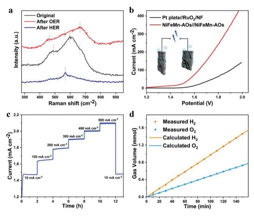
Fig. 5 (a) Raman spectra of the NiFeMn-AOs sample. (b) Polarization curves of NiFeMn-AOs//NiFeMn-AOs and Pt plate//RuO<sub>2</sub> electrolyzer (without iR-compensation). (c) Chronopotentiometry curves of NiFeMn-AOs//NiFeMn-AOs at various current densities. (d) The volumes of  $H_2$  and  $G_2$  experimentally measured at 100 mA cm<sup>-2</sup>.
