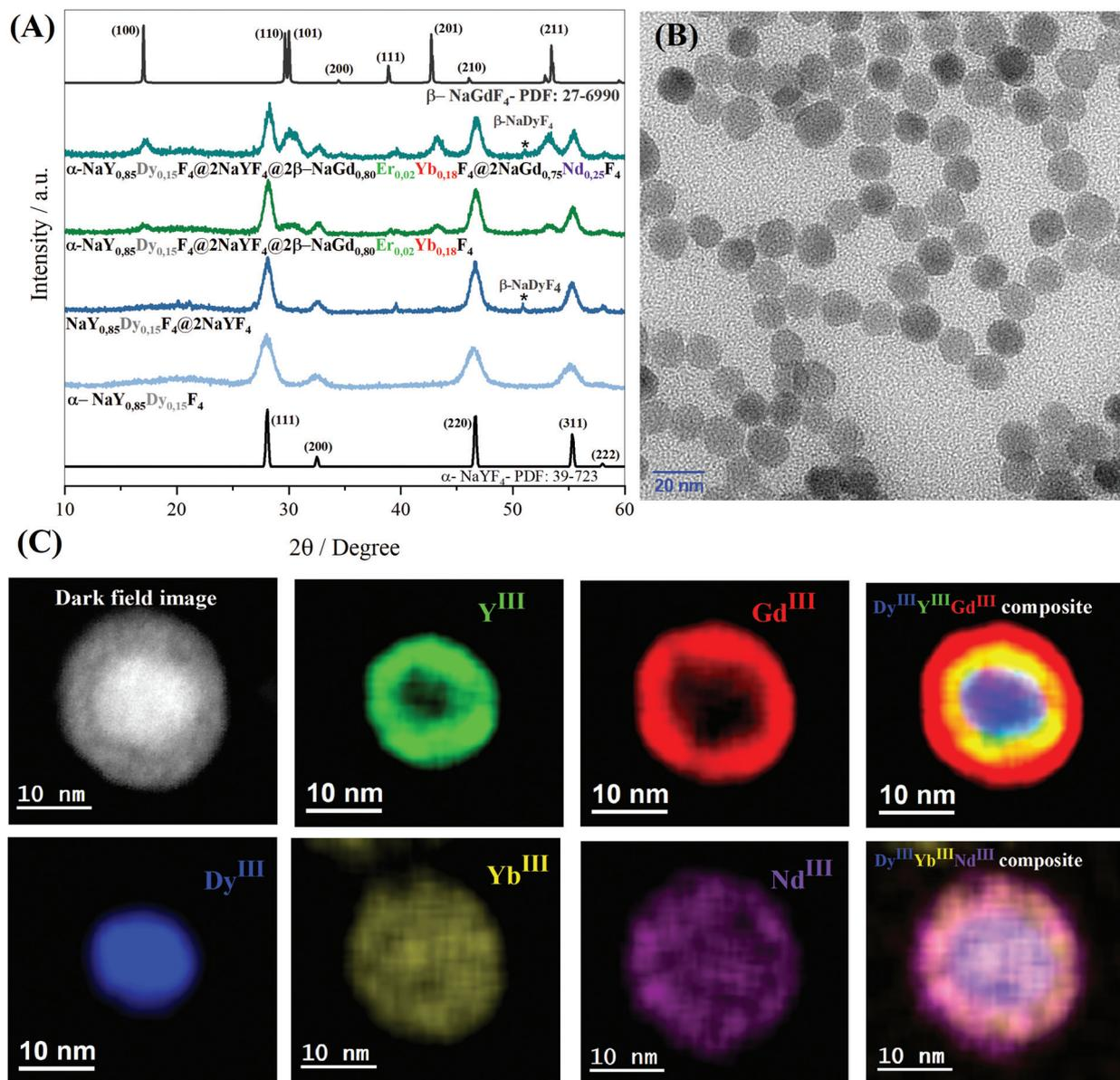
Fig. 2 (A) P-XRD data compared with references:  $\alpha$ -NaYF<sub>4</sub> (PDF no. 77-2042) and  $\beta$ -NaYF<sub>4</sub> (PDF no. 16-334). (B) Bright field TEM image. (C) EDS elemental mapping of the  $\alpha$ -NaY<sub>0.85</sub>Dy<sub>0.15</sub>F<sub>4</sub>@ $\alpha$ -NaYF<sub>4</sub>@ $\beta$ -NaGd<sub>0.80</sub>Er<sub>0.02</sub>Yb<sub>0.18</sub>F<sub>4</sub>@ $\beta$ -NaGd<sub>0.75</sub>Nd<sub>0.25</sub>F<sub>4</sub> nanoparticle.
