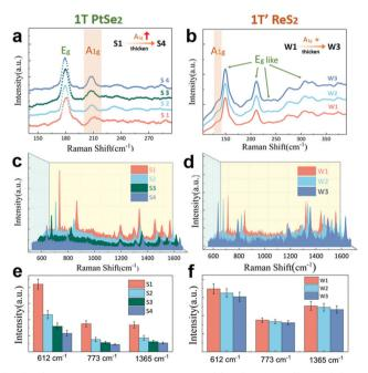
Fig. 5 Characteristic Raman spectra of (a)  $PtSe_2$  films (S1 to S4) and (b)  ${\rm ReS_2}$  films (W1 to W3). Enhanced Raman spectra of  ${\rm 10^{-5}~M~R6G}$  on the (c) PtSe<sub>2</sub> films (S1 to S4) and (d) ReS<sub>2</sub> films (W1 to W3). The extracted average signal intensities integrated at 612 cm<sup>-1</sup>, 773 cm<sup>-1</sup> and 1365 cm<sup>-1</sup> for S1 to S4 (e) and W1 to W3 (f).
