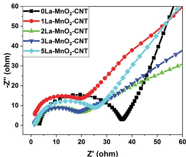
Fig. 11 EIS spectra of undoped and La<sup>3+</sup>:MnO<sub>2</sub>-CNT nanohybrids.
