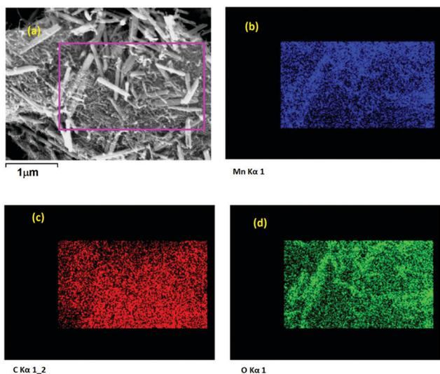
Fig. 4 FESEM (a) and elemental maps of (b) Mn; (c) C, and (d) O for 0La-MnO<sub>2</sub>-CNT.
