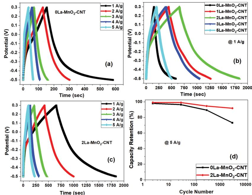
Fig. 9 GCD profiles of 0La-MnO<sub>2</sub>-CNT at different constant current densities (a); comparative GCD profiles of undoped and La<sup>3+</sup> MnO<sub>2</sub>-CNT nanohybrids at 1 A g<sup>-1</sup> (b); GCD profiles of 2La-MnO<sub>2</sub>-CNT at 1 A g<sup>-1</sup> (c); cycle stability of 0La-MnO<sub>2</sub>-CNT and 2La-MnO<sub>2</sub>-CNT at 5 A g<sup>-1</sup> up to 5000 cycles (d).
