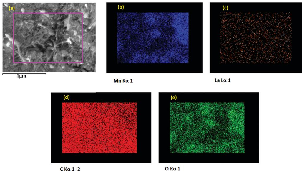
Fig. 5 FESEM (a) and elemental maps of (b) Mn; (c) La; (d) C; and (e) O for 2La-MnO<sub>2</sub>-CNT.
